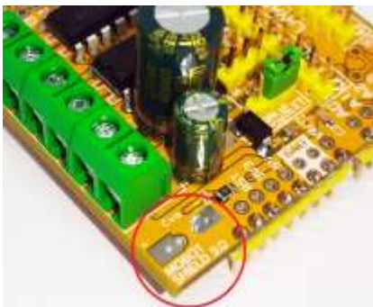
Capacitor slot for the motor power line
