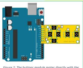
Figure 2: The buttons module mates directly with the Arduino pins 8~13 and GND and may be connected without wiring
