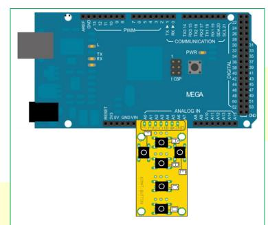
Figure 6: Direct Connection with Arduino Mega pins A0~A5 and with pin A6 used as ground. Set A6 as Output and initialize it to LOW state
