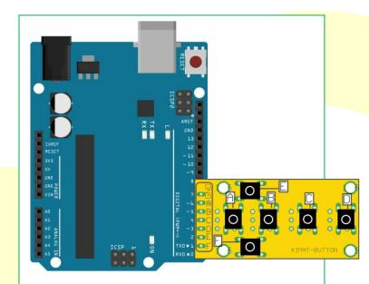
Figure 4: Connecting to other consecutive pins without wiring
