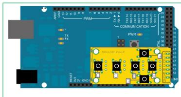
Figure 5: Direct Connection with Arduino Mega pins 42,44,46,48,50 and 52 and GND pin
