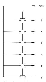
Buttons A~D are latching pushbuttons while buttons E and F are momentary pushbuttons.
