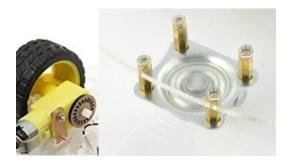
The caster wheel is installed with the brass stand offs.
