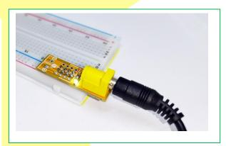
There are additional 4-pin header slots for the positive and negative terminals where the user may install extra pin headers in either the top or bottom side of the PCB. The module accepts continuous voltages between 3V and 12V and surges up to with a current of up to 1A. The module has a built-in power LED indicator.
