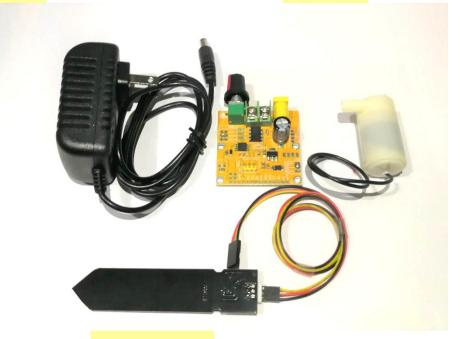
The pump-based kit comes with an irrigator controller board, a DC power supply, a capacitive soil moisture sensor, and a submersible water pump. The image below shows the proper wiring of the submersible water pump to the irrigator controller board terminals.
