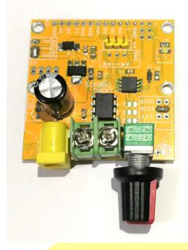
The Layad Circuits One Channel Irrigator also makes sure that proper delays and rest periods for the valve or pump are observed during operation to prevent damage. The built-in potentiometer allows the user to adjust the moisture level threshold value at which the valve or pump is activated and deactivated. The on-board heartbeat LED indicates that the device is
