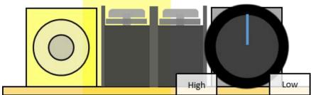
When the threshold adjustment knob is at the LOW position, the device will irrigate ONLY when the soil moisture level being detected by the soil moisture sensor is LOW. When the threshold adjustment knob is at the HIGH position, the device will irrigate even if the soil moisture level being detected by the soil moisture sensor is HIGH. Set the threshold knob to anywhere in the middle to irrigate when the optimum level of soil moisture level is reached.
