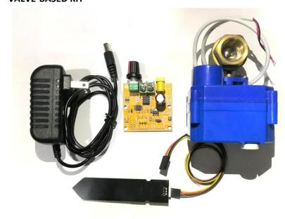
The valve-based kit comes with an irrigator controller board, a DC power supply, a capacitive soil moisture sensor, and an electronically controlled valve. The image below shows the proper wiring of the valve to the irrigator controller board terminals.
