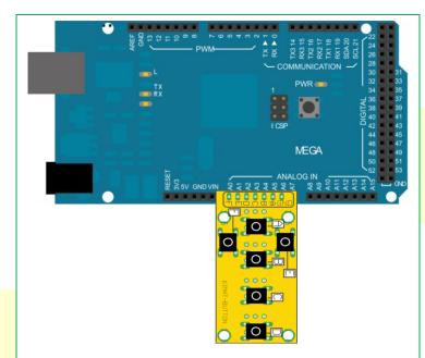
Figure 6: Direct Connection with Arduino Mega pins A0~A5 and with pin A6 used as ground. Set A6 as Output and initialize it to LOW state
