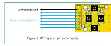
If you are connecting to pins that are consecutive, you could also use a digital pin as ground by declaring that pin as output and setting it LOW.
