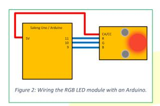
Usage of the module is straight forward. Connect each color pin to a digital pin on the microcontroller. For a CA board, connect the CA/CC pin to 5V. For CC variants, connect this pin to GND. Turn each color on and off a high or a low respectively. Generating PWM signals on each color pin produces more colors.
