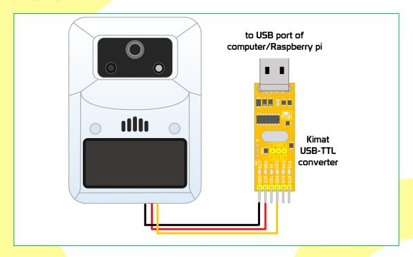
Once connected the data can be read out of the serial port (COMx in Windows) set at a baud rate of 9600, 8 databits, No parity and 1 stop bit. Program the application software to receive this data and process or present it accordingly. This computer/Raspberry Pi application is beyond the scope of this document.
