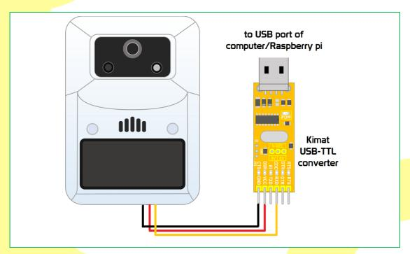
Once connected the data can be read out of the serial port (COMx in Windows) set at a baud rate of 9600, 8 databits, No parity and 1 stop bit. Program the application software to receive this data and process or present it accordingly. This computer/Raspberry Pi application is beyond the scope of this document.
