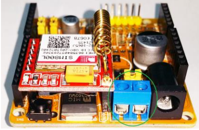
Figure 13: Add a terminal block as power connector
