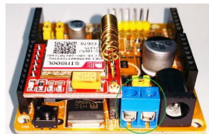
Figure 13: Add a terminal block as power connector
