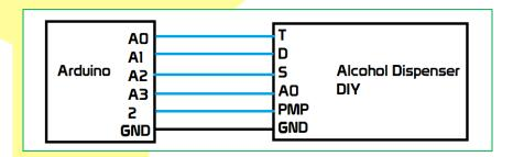
Analog output of Alcohol dispenser T, D, S and A0 are connected to analog pins A0, A1, A2 and A3 of Arduino. The digital input of the Alcohol dispenser is connected to output digital pin 2 of Arduino.
